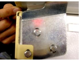
Reinsert all 3-freezer hinge bolts finger tight. Ensure the gap between the freezer door and refrigerator door is uniform and then tighten the screws.
